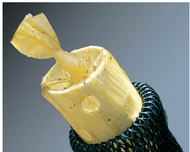
Figure 7. Discoloration of dialysis sampler membrane after 2 weeks of deployment in a well, Hickam Air Force Base, Hawaii, July 2001.
