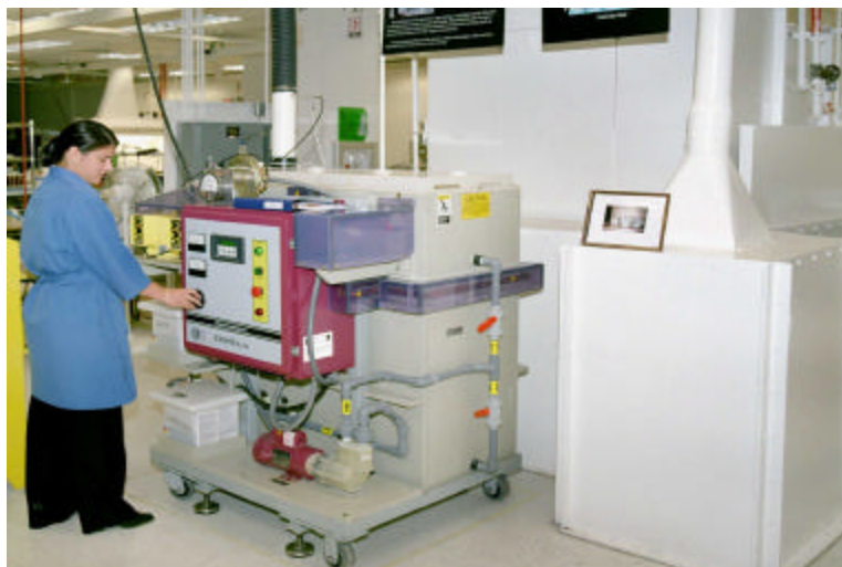
"E-floter" on a waterfall lacquer paint booth in the TOW missile line.
