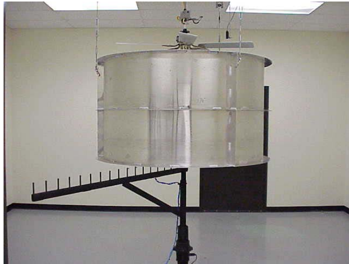
Figure 3.7 – Testing Cylinder, Actuator, and Sensor Rotating Arm
