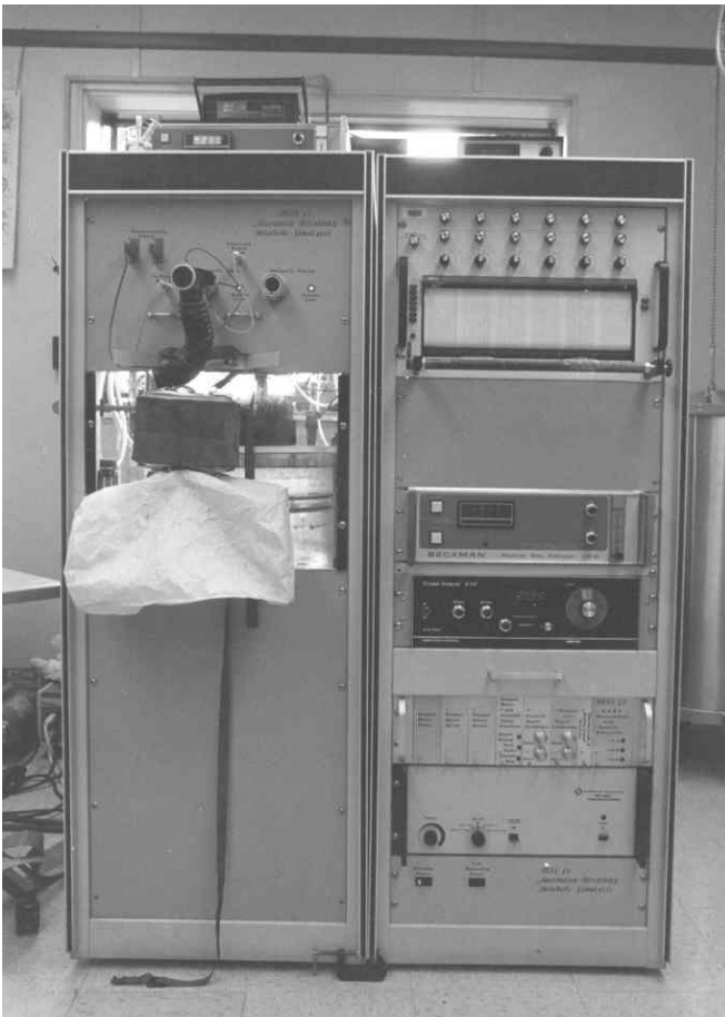
Figure 1.—Breathing and metabolic simulator.
