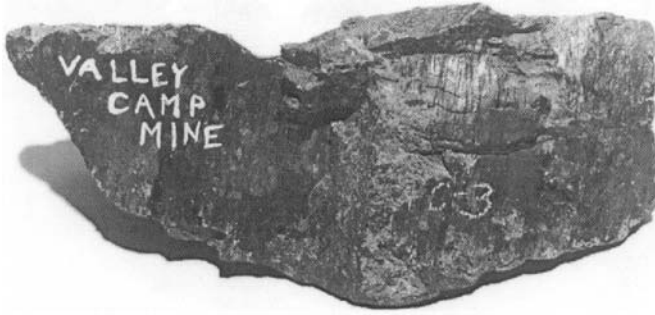
Figure 26.—Slickensides on a rock fallen from a coal mine roof.
