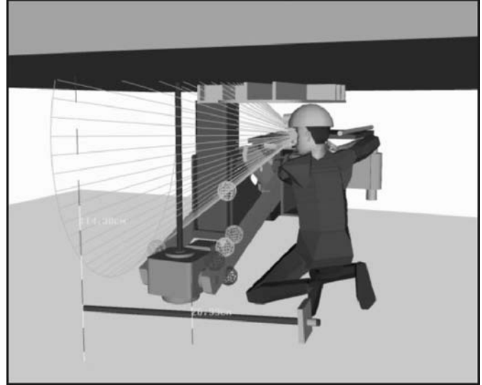
Figure 9.–Virtual operator's behavior hand off drill and boom arm.
