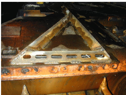
Figure 11. 1/2 inch angle iron antenna.
