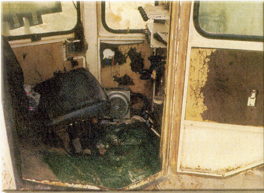
Figure 4: A ¼- to ½-in.-thick layer of gritless, canola oil-based sweeping compound was spread on the floor of the enclosed cab during three shifts.
