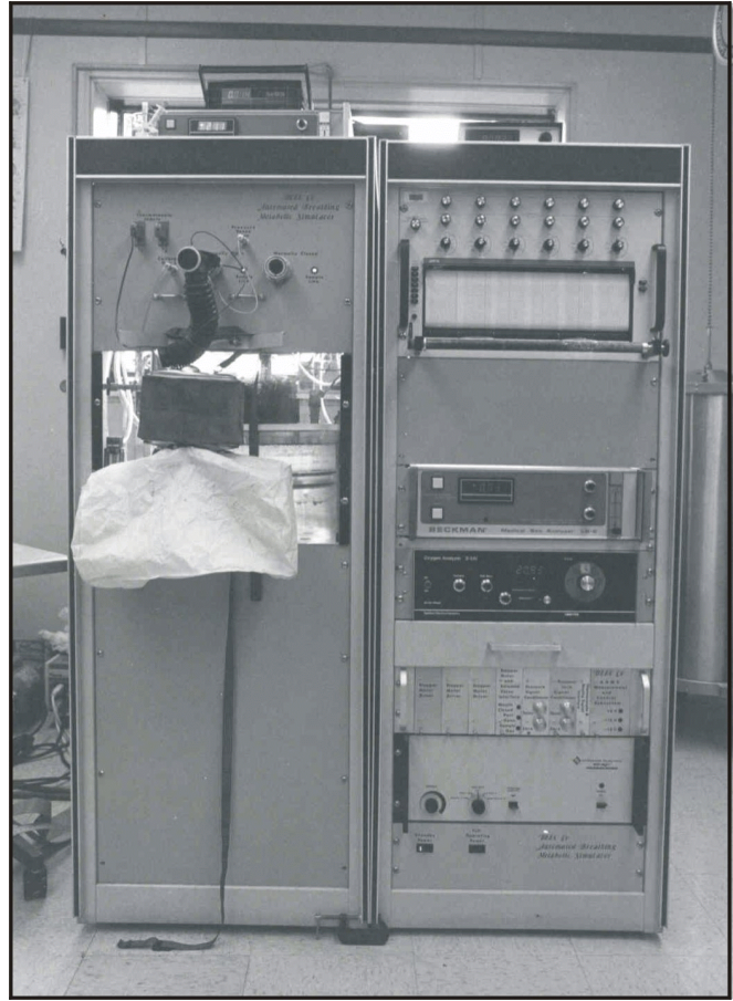
Figure 1.—Breathing and metabolic simulator at the NIOSH Pittsburgh Research Laboratory, Bruceton, PA.
