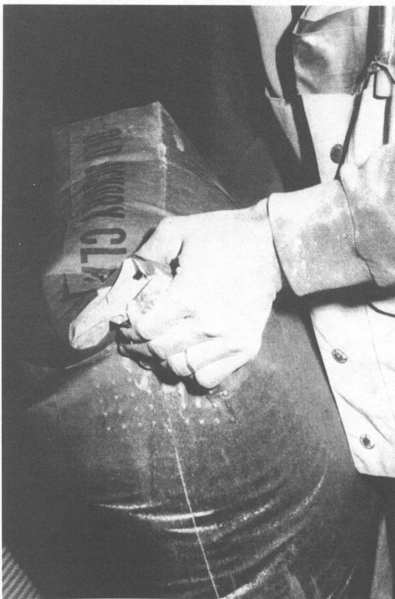
FIGURE 15 Bag operator crimping bag valve closed after removing bag from fill nozzle.
