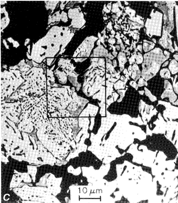
Figure 21.—Electron probe photographs of pre- and postinduration oxidized fluxed (batch 7) pellets. A , Preinduration composite; B , preinduration X-ray elemental maps; C , postinduration composite; D , postinduration X-ray elemental maps.
