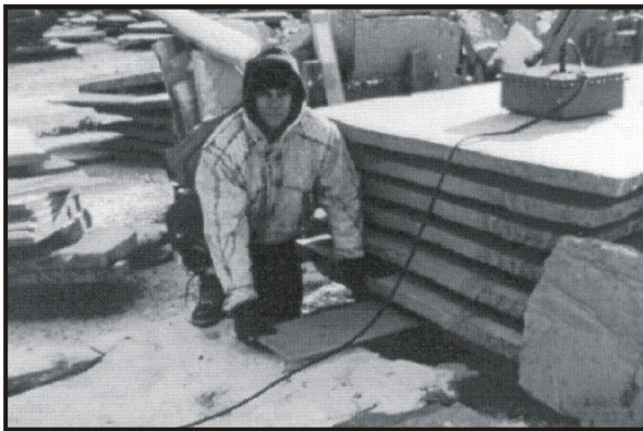
Figure 3.—Collecting GPR data from a 900-MHz antenna through a stack of sandstone slabs.
