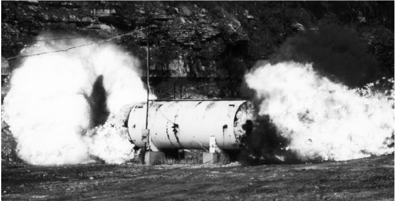
Figure 30—Coal dust ignited by unstemmed ANFO at the Lake Lynn cannon gallery showing flame exiting from both ends. (Photo by Kenneth L. Cashdollar, Pittsburgh Research Center.)
