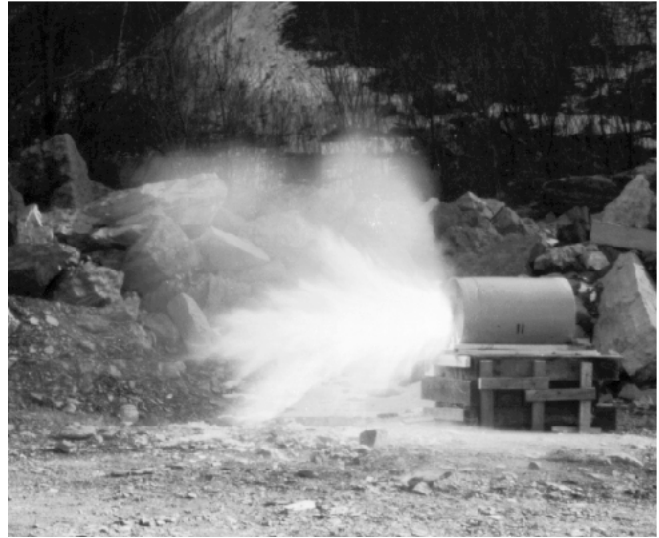
Figure 29.—Flame exiting from cannon after detonation of blasting agent. (Photo by Kenneth L. Cashdollar, Pittsburgh Research Center.)
