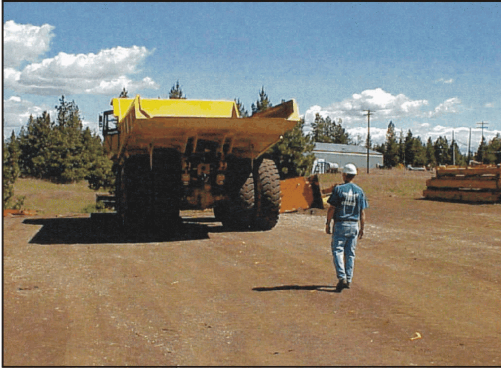
Figure 7.—Test configuration using person as obstacle.
