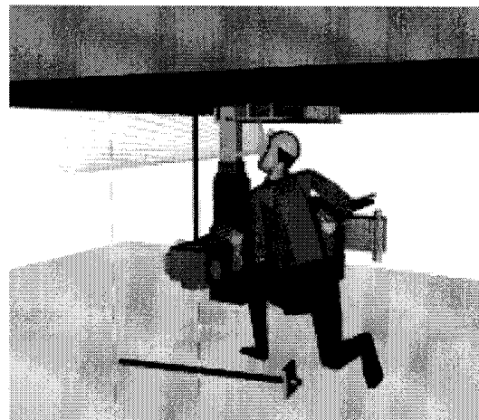
Figure 4b. Operator's risk behavior, hand on boom arm
