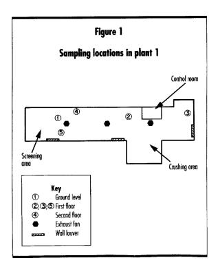
sampling locations were chosen to provide a good dust profile of the plant.
