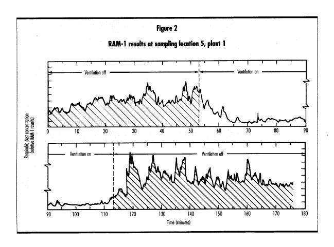
Table I lists dust concentration reductions determined by both the gravimetric dust samplers and RAM-1s at each location. The results are based on comparing average dust concentrations when the ventilation system was on with those when it was off. The overall average reduction for the five locations was about 40 percent (although the correlation between the two instruments at each location was less than expected).
