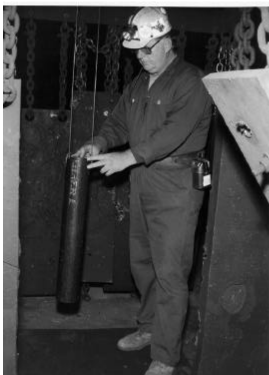
Figure 3. Blasting agents were confined in a 27-inch (69-cm) length of 4-inch (10-cm) Schedule 80 steel pipe.
