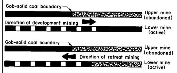
Studies show that stress in the lower mine pillars can be reduced when you are mining beneath a gob-solid coal boundary in a overlying mine by following two design criteria: (1) Develop pillars from the solid to the gob side of the boundary, and then retreat pillars from the gob to the solid side, and (2) support the boundary edge with a row of pillars.
