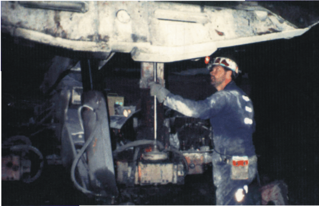
Figure 1.—Bolter operator beginning drilling procedure.
