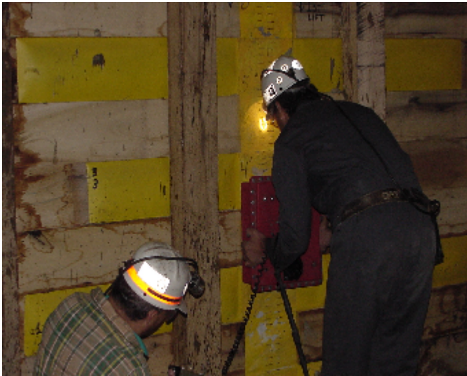
Figure 9. Researchers performing GPR scan of mine seal.
