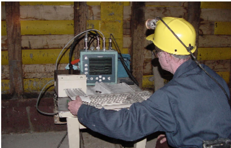
Figure 8. Engineer monitoring SIR-2 unit during GPR scan of mine seal.
