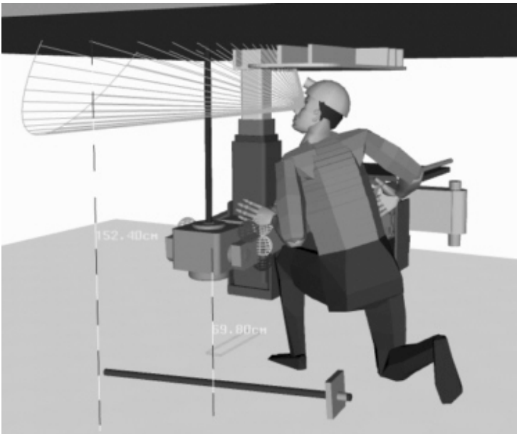
Figure 2. Vision cone in the roof bolter model
