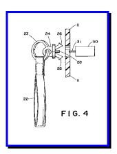
Referring next to FIG. 4, wherein the cut-away portion of FIG. 2 is shown in an enlarged view, the key 24 is shown detached from housing 11. As seen in FIG. 4, the spring loaded plunger 31 of switch 30 is permitted to slidably extend into its unactuated position in the absence of key 24 and associated centrally located fixed plunger 28. FIG. 4 shows the pair of barbed, springy legs 26 in their unsprung position and ready for reinsertion into the housing 11 to re-enable
