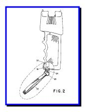
Referring now to FIG. 2, a portion of the housing 11 is shown cut-away. The key 24 is shown received into the housing 11 and in contact with plunger 31 of switch 30. The switch 30 is fixed mechanically to a
