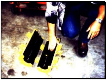
San Diego substituted an automated lubrication system that is more cost-effective and reduces the risk of injuries. The annual cost of the manual process exceeded \$320,000, while the yearly cost of the automated system is approximately \$34,000. This ergonomic intervention resulted in more than a ninefold reduction in cable cleaning and lubrication costs in addition to the reduction in the number of hand injuries.
