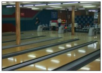
bowling balls hit the pins. Noise levels above 84dB(A) are considered hazardous by the DOD. The Rota Industrial Hygiene surveys used ambient sound level meter and personal noise dosimeter workplace monitoring that identified pinsetter mechanics for full entry into the Naval Station Rota Spain hearing conservation program.
