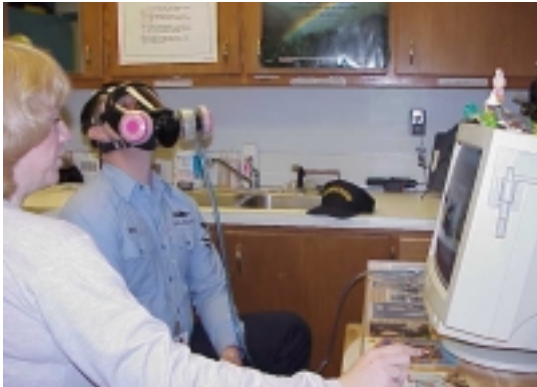
Safety specialist using dedicated quantitative fit testing unit to prepare sailor for respirator use.
