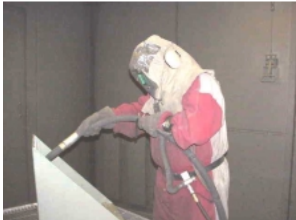
Wearing sandblast air line respirator in walk-in booth.
