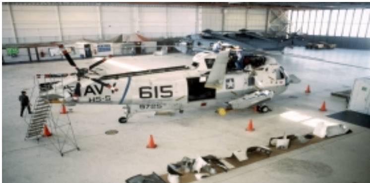
SH-3C Sea King helicopter being prepared for corrosion inspection inside hangar
