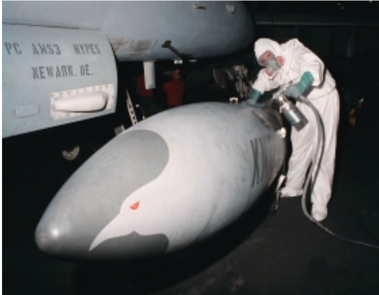
Aircraft spray painting operation inside hangar.
