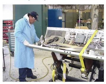
Aircraft door is held by fixture allowing sheet metal mechanic to work in neutral posture while using low vibration powered hand tool.
