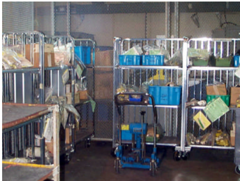
Staging and transfer carts accommodate aircraft parts and fold up for easy storage
