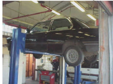
Inspected items include brakes, tires, lights, turn signals, seat belts, and horns
