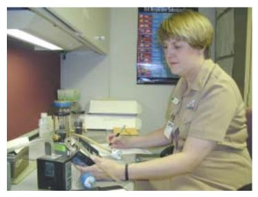
Industrial hygienist calibrates equipment used to measure airborne concentrations of health hazardous substances
