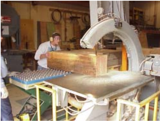
Shipwrights using rollertop hydraulic lift table no longer have to support weight of keel blocks
