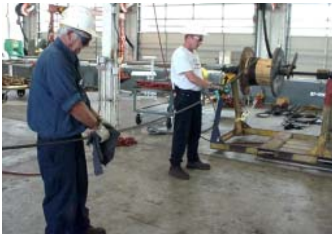
Manually cleaning and lubricating wire rope from a spool required riggers to stand and use repetitive motions for long periods
