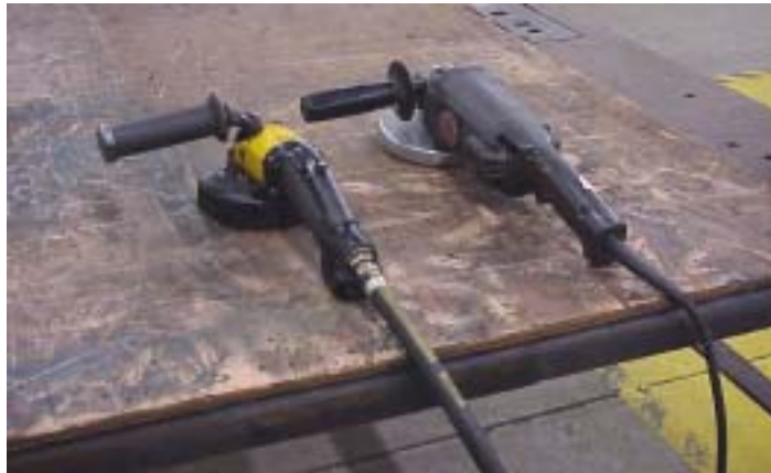
Lightweight, pneumatic grinder on left produces far less vibration than heavy, conventional grinder on right
