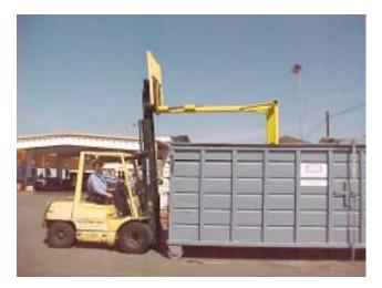
Remote controlled *hazardous waste rake* prevents slips, trips, falls, back injuries, and risk of contact with wastes
