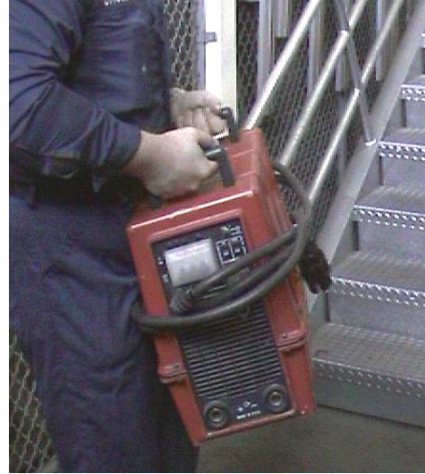
Welders reported muscle discomfort after carrying the 70 pound power-con
