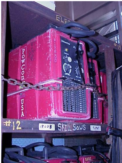
Power-cons provide electricity for portable welding operations
