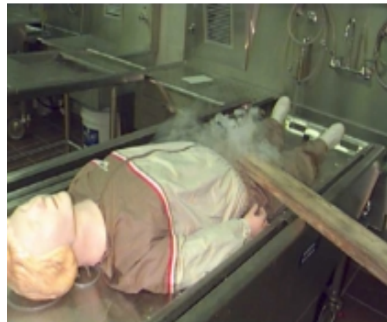
NFESC smoke test demonstrates capture of vapors at autopsy table local exhaust system
