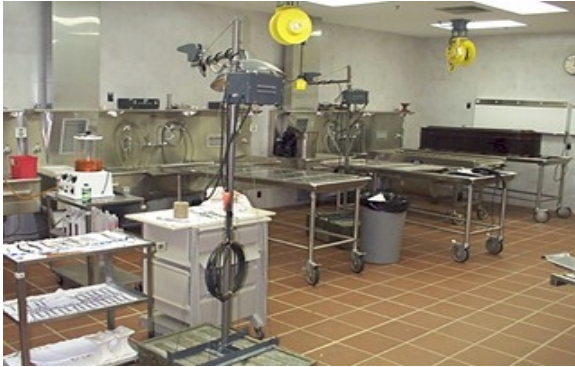
Original autopsy room had general ventilation system with 12 room air changes per hour
