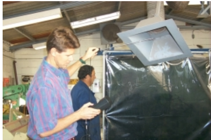
NAVHOSP Rota Industrial Hygienist performs Local Exhaust Ventilation system airflow evaluation in feet per minute and meters per second for Industrial Hygienist reports at locations where there are Spanish workers
