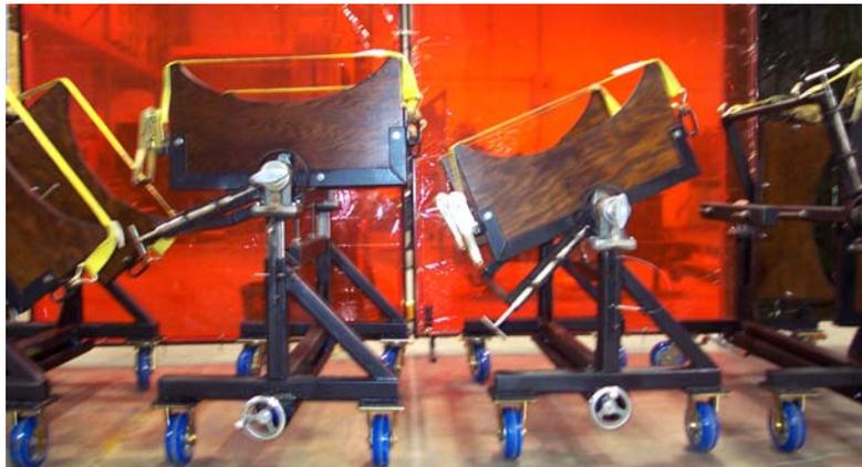
**Door fixtures lock aircraft doors in place for stability; fixtures also rotate and are height adjustable, allowing worker comfort during repairs**
