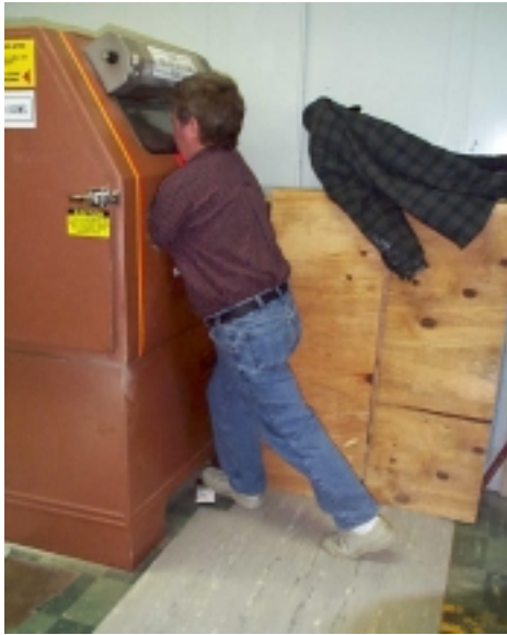
Workers of above- or below-average height had to adopt awkward postures to use the blast cabinet
