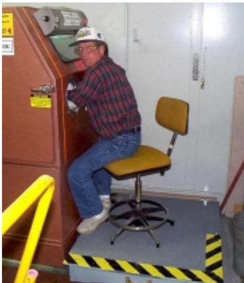
Workers have more flexibility to comfortably sit or stand using the foldaway platform
