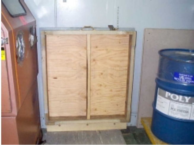
Space saving foldaway platform provides ergonomic comfort for blast cabinet workers
