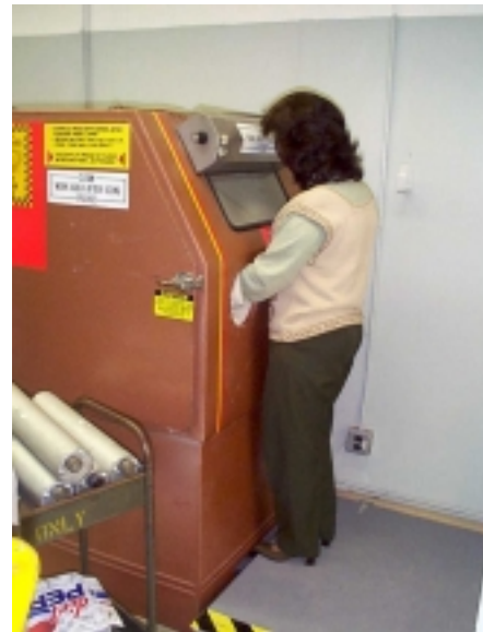
Foldaway platform eliminates awkward postures while using blast cabinet
