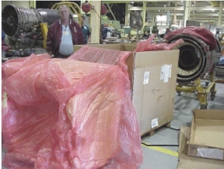
Cutting open shipping carton releases suction so workers can easily slide out combustion liner
