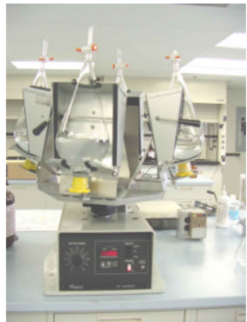
Automatic separatory funnel shaker eliminates shaking by hand
