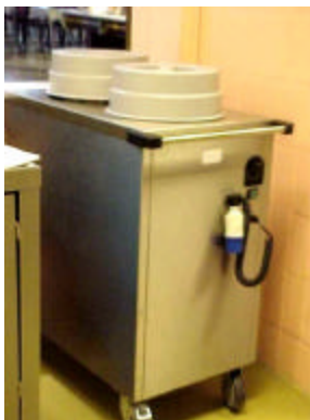
Self-actuating carts eliminate bending to pick up dishes
