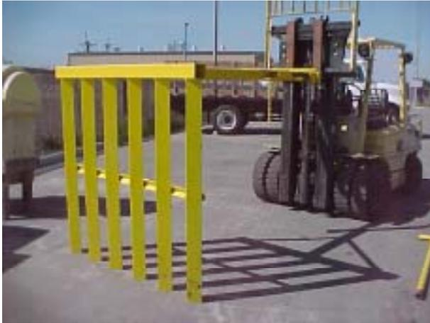
**Remote control Hazardous waste rake attached to forklift redistributes hazardous waste inside roll-offs**
