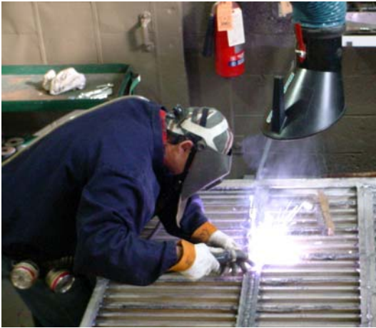
Articulating arm allows welder to easily maneuver parts for welding under air extraction unit
