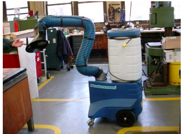
Portable air extraction unit is used for welding tasks performed on site.
