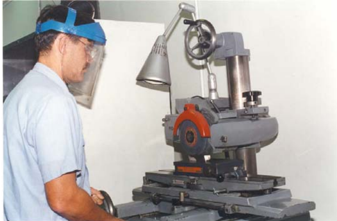
Safety requirements for metalworking at NAS Sigonella include eye and face protection.
