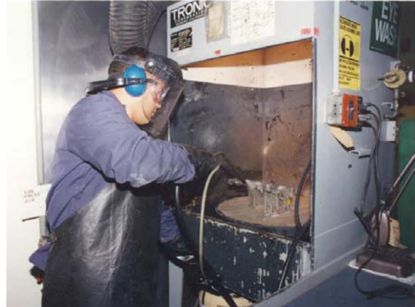
Use of pressurized hand spray tools at NAS Sigonella requires proper ventilation and eye, face, skin, and hearing protection.
