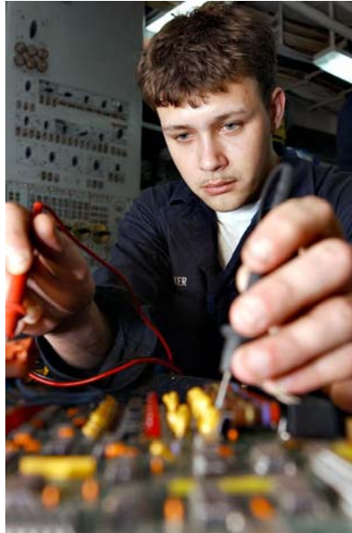
Interior Communications Electrician troubleshoots a faulty component on an over-speed trip panel circuit card from the number 4 Main Machinery Room aboard USS Kitty Hawk.
