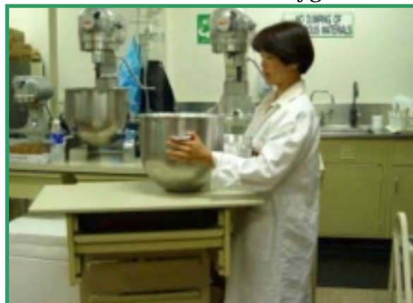
Full bowls of lotion are transported to the scissors lift table via a wheeled cart
