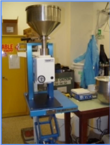
Hydraulic scissors lift table is permanently fastened to the floor with lotion dispenser mounted on top
