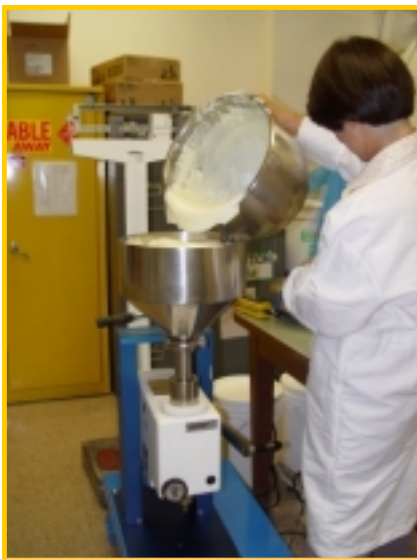
Hydraulic scissors lift table can be lowered for transfer of lotion into the hopper
