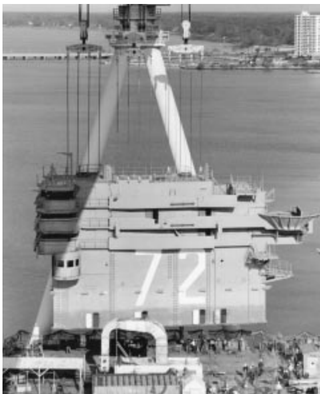
Abraham Lincoln gets her island during construction.
