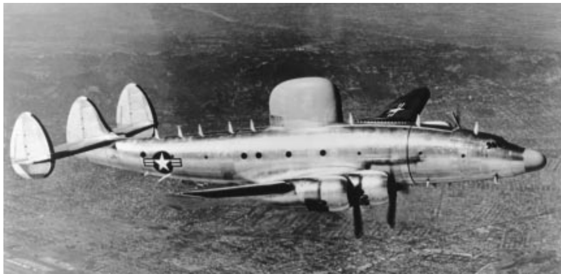
Early version of Lockheed WV, radar picket plane for long- range patrol, on seaward exten- sion of Dewline 1053793
