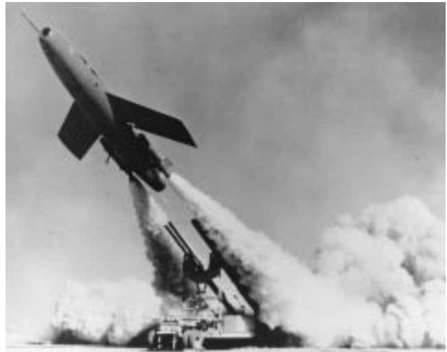
Test of Regulus I surface-to-surface missile, JATO launches Bird and main engine provide long range 1053792
