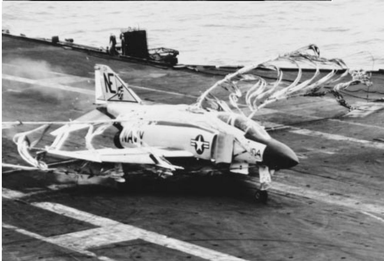
*F-4J Phantom of VF-21 making a successful barricade arrested landing aboard Ranger.*
